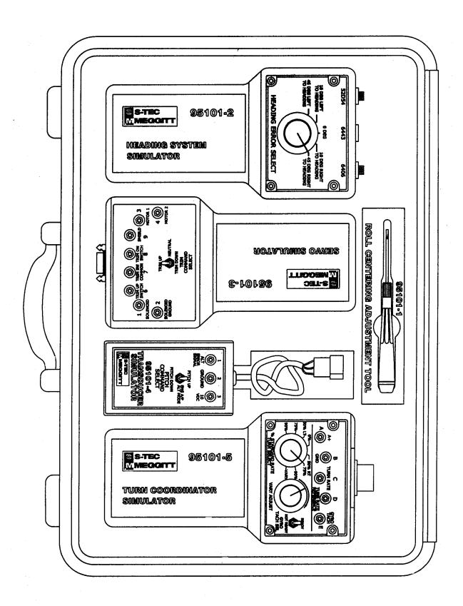
Fig. 1-1. Flight Line Autopilot Tester
