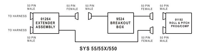
Fig. 1-2. Breakout Connections
