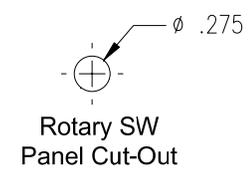
NOTE: Not to scale, Units=Inches unless otherwise specified. Square Mount requires separate mounting of Mute/Repeat and Rotary Switches
