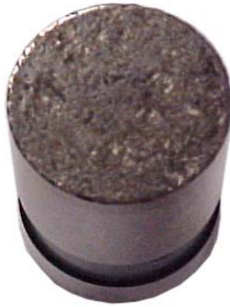
FIGURE 9 REPLACEMENT SIGNATURES, SPALLED LIFTER
