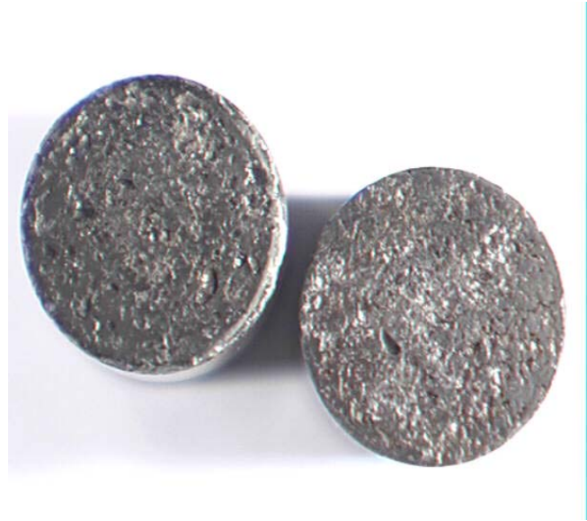
FULL FACE SPALLING
