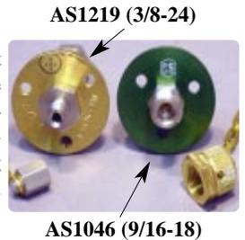
The TA-380-S & -N are for the MS22066 & MS22035 filler ports. The TA-916-S & -N are for the 9/16-18 'SCOTT' fittings. The -N is for nipple and the -S for 'SOCKET' on the CGA-540 ends. This nomenclature is used because the term Male/Female was constantly being confused with CGA fittings. Micro-particle filters are installed on the 540 ends and an O-ring is on the 540 nipple for an air-tight fit by hand.
