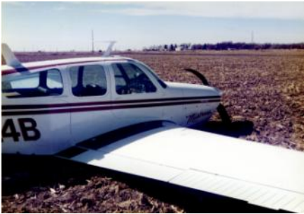
No damage to any control surfaces
