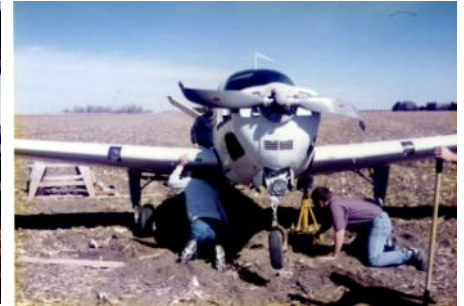
Dug holes beneath wheels, then lowered. Made ramps with boards so could pull out
