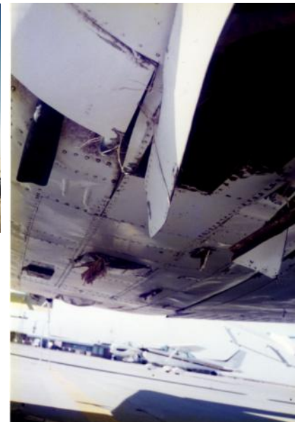
Damage, did need new nose gear doors
