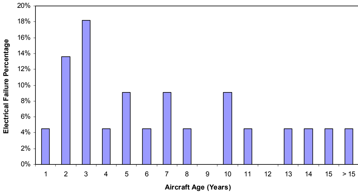
FIGURE 14. ELECTRICAL FAILURE PERCENTAGE VS AIRCRAFT AGE
