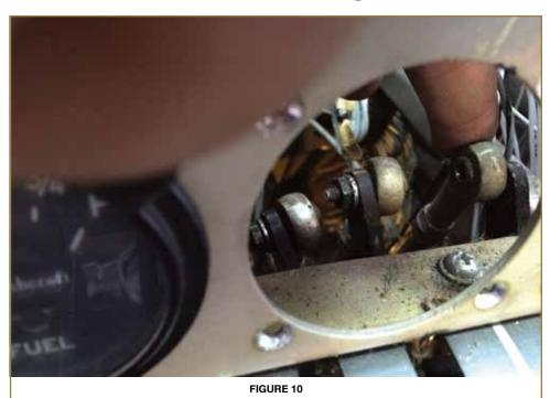
Other critical cable placements and hold-down positioning in the engine bay and the interior blocks include the positioning of idle/mixture cut-off for the throttle and mixture cables, and full RPM and feather for the props. In my experience, leaving the console open until you are nearly finished is a good idea. This will allow you to make the final feather adjustments for cable throw, and use the interior holddown block for any final positioning
