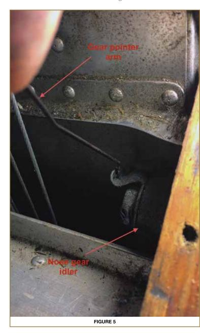
Another area of caution is the landing gear pointer indicator (if your aircraft is so equipped). **Figures 5**, **6**, **and 7** show the little arm that connects the pointer arm to the nose gear idler arm such that when the nose gear rod is pushed forward, the rod transfers this motion into a motion that pulls on the pointer arm.
