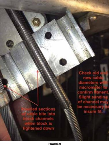
The inside cables are held in place by a pair of aluminum blocks that are fastened to the console framework. **Figure 8** shows the block's fasteners and **Figure 9** shows the hold-down block itself. The grooves in the block form a clamping force around the knurled section of the cable and the console frame arm. These fasteners are small and quite old so you might consider sourcing new ones especially if the Phillips heads start to show any signs of destruction.
