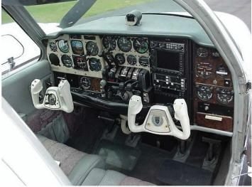
All 55-series Barons share the same panel layout and power and flight controls arrangement, with optional dual controls (pictured) or a standard, throw-over control column.
